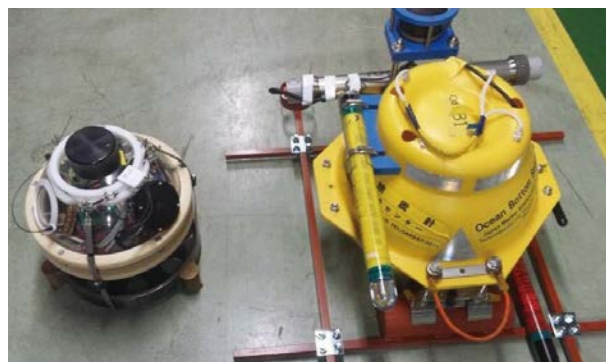
Figure 3. Left: newly developed next-generation OBS, right: conventional OBS
