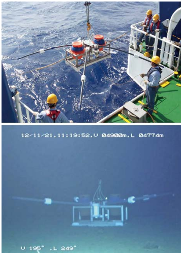
Figure 3. (Top) Deployment of the Vector Tsunami Meter (VTM) from KAIKEI . (Bottom) VTM on the seafloor photographed by KAIKO 7000II
