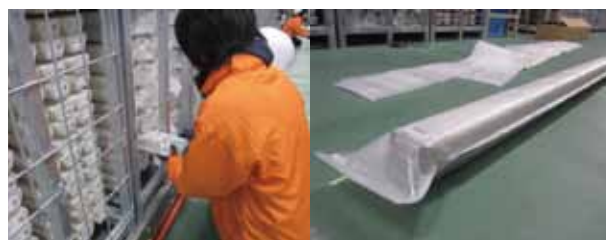
Photo 2. Packing work (left) and a packed core sample (right)
