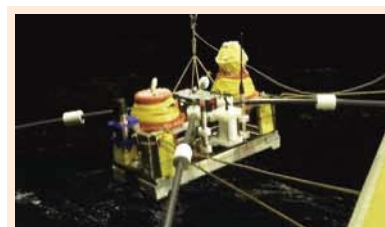
A new ocean-bottom tsunami monitoring methodology with Vector TsunamiMeter was tried out.
