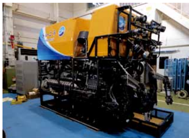
Figure 1. Kaiko Mk-IV : Heavy ROV for seafloor resource exploration
