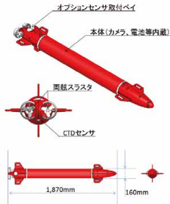
図:氷縁域観測用小型AUV試作機 Figure: Compact AUV prototype capable of short-range monitoring of marine environments under the sea ice
