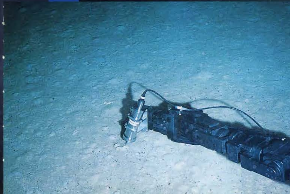
Measuring heat flow.
