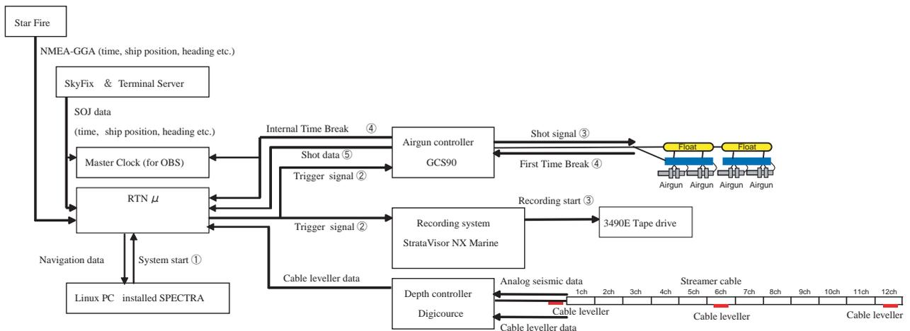
Figure 6: Flow chart for the MCS recording system. Circled numerals show the timing flow of this seismic system.
