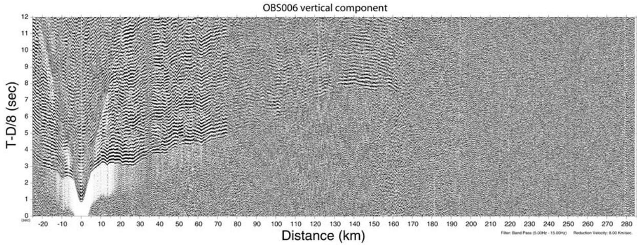
Figure 7: Vertical record section recorded by OBS#6. All traces are filtered by 5-15 Hz. Vertical and horizontal axes are offsets from OBS and reduced traveltimes by 8 km/s.
