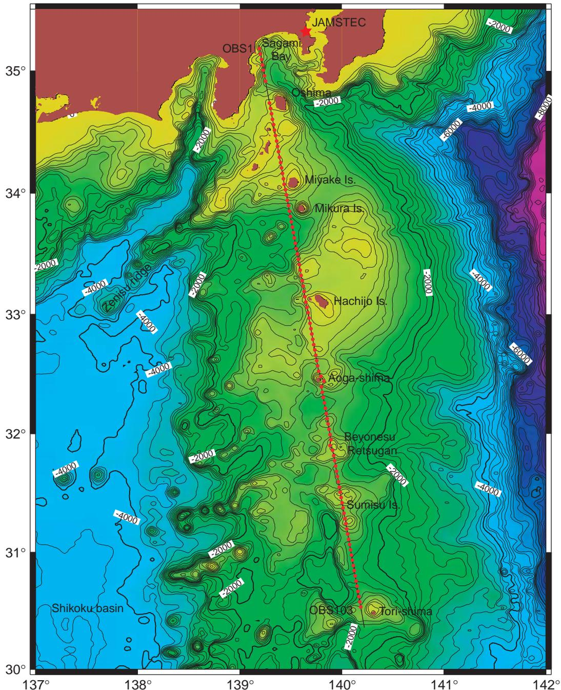
Figure 1: Map of the experimental area. Solid circles indicate OBSs. We shot an airgun array on a thick black line.
