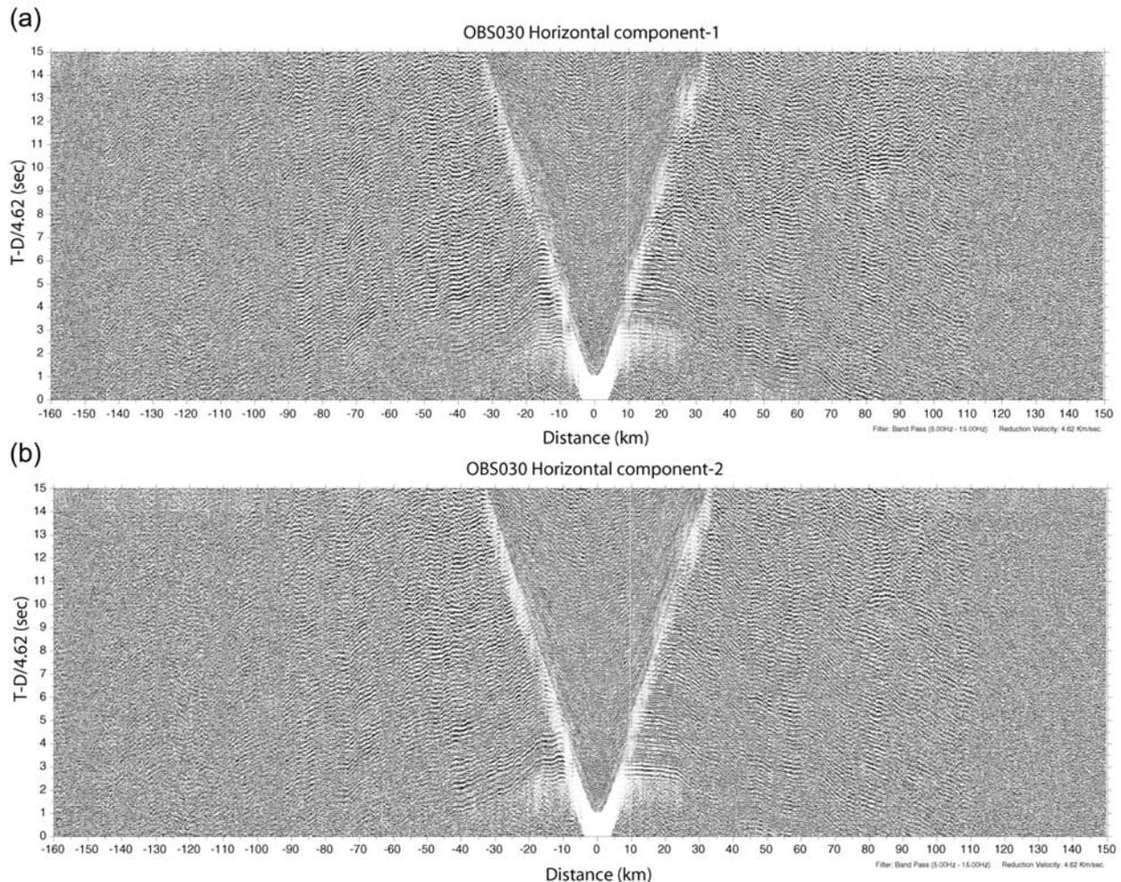
Figure 10: Horizontal record sections recorded by OBS#30. All traces are filtered by 5-15 Hz. The reduced velocity is 4.62 km/s. (a) Horizontal component-1. (b) Horizontal component-2.
