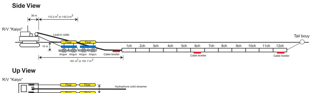
Figure 4: Geometry of airgun system and the hydrophone streamer.
