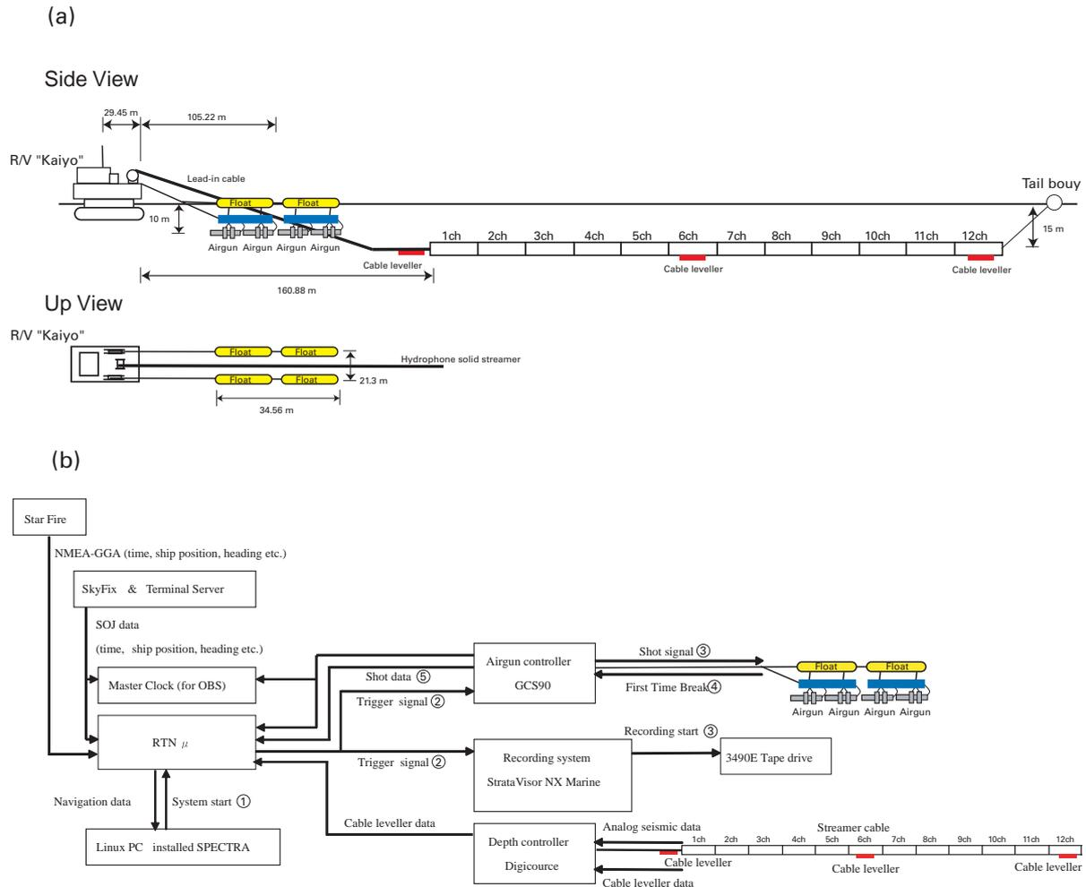
Figure 4: MCS system (after Takahashi et al., 2005). (a) Geometry of airgun system and the hydrophone streamer. (b) Flow chart for the MCS recording system
