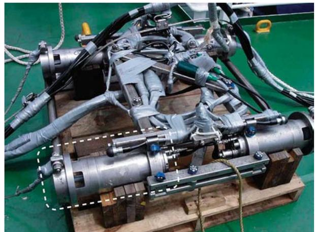
Figure 5: Photograph for G-gun array. G-gun array is composed of four 150 cu. in. G-guns fixed with a metal frame. White dotted rectangle shows a G-gun.
