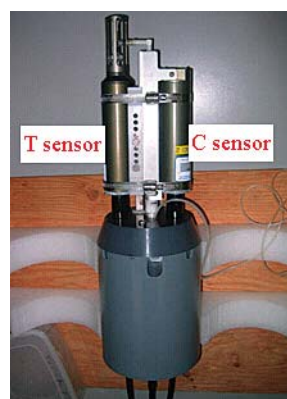
Figure 3: Standard sensor unit of temperature (SBE3; T sensor) and conductivity (SBE4; C sensor). A water pump (SBE5) is attached to SBE4 to circulate seawater in C sensor cell.
