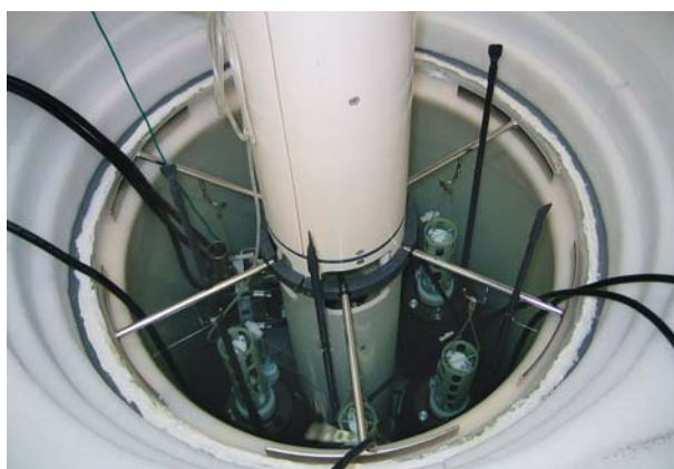
Figure 4: Bath with a reference sensor unit and five SBE41s.
