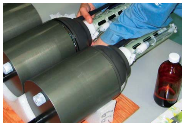
Figure 2: Preparing SBE41s of Apex floats to set them on the calibration system.
