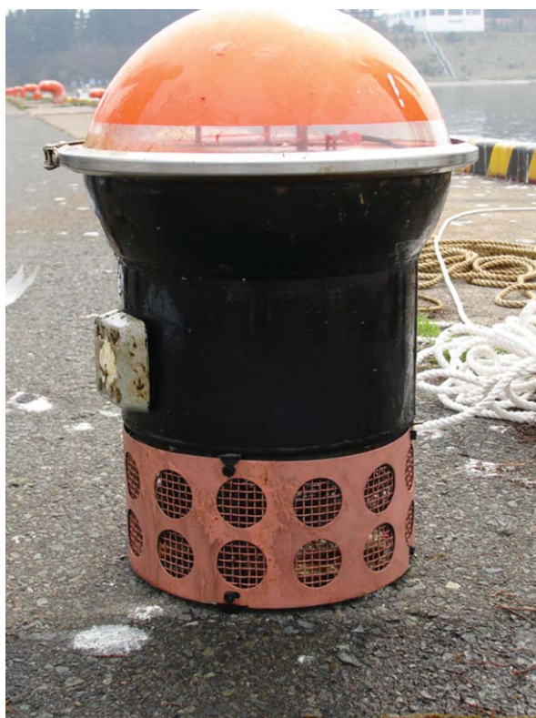
Fig. 3. Drifting buoy system with sea surface p\text{CO}_2 sensor. The silicon-based antifouling paint (CMP Bioclean C, clear and colorless) was used as biofouling prevention for the surface (black portion) of our drifting buoy system. The black color of the surface is from the epoxy resin paint (under coat).
