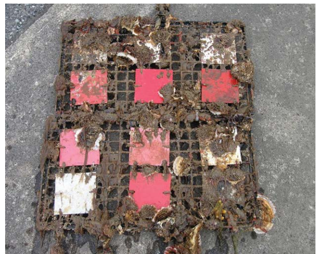
Fig. 2. Results of antifouling tests. See Table 1 for antifouling paints used. The plate-1 is the control (aluminum plate only) without antifouling paint.
