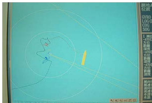
Fig. 2. Monitor screen of the acoustic navigation system installed aboard R/V Mirai . We can confirm the positions of R/V Mirai and the transponder.
