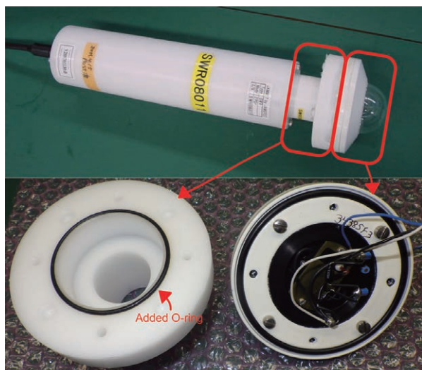
Fig. 9. Overview of shortwave radiation sensor and housing structure.
