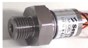
Fig. 10. Pressure transmitter using silicon strain gauge.
