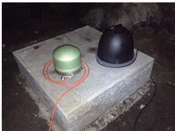
Fig. 3. Broadband seismological station CHUK in Chuuk island.
