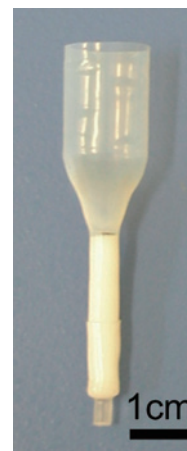
Fig. 1. Handmade PFA column with resin volume of 0.2 ml.
