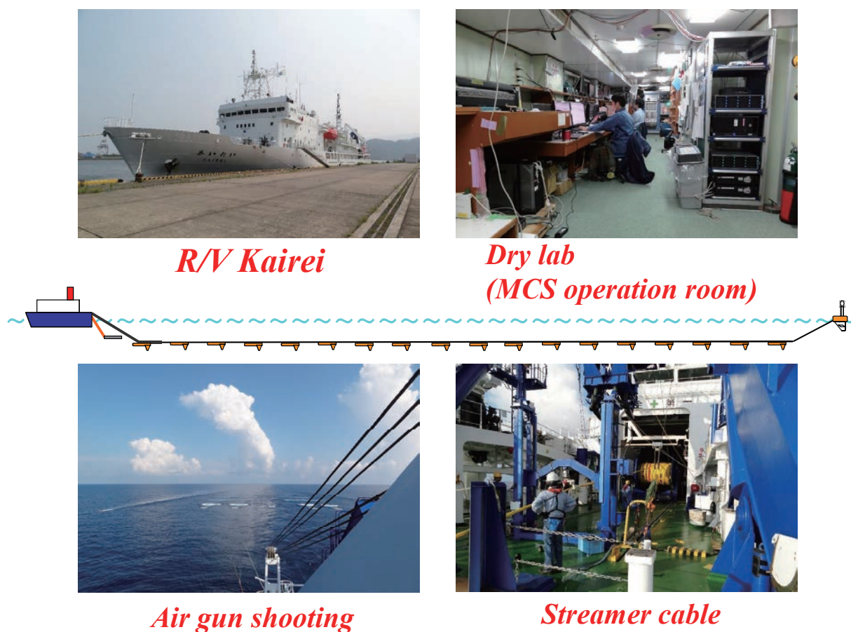
Fig. 2. MCS system aboard the R/V Kairei which acquired our data. For details of the R/V Kairei , refer to JAMSTEC (2018), and for more detail of the MCS system, refer to Miura (2009) and JAMSTEC (2017).
