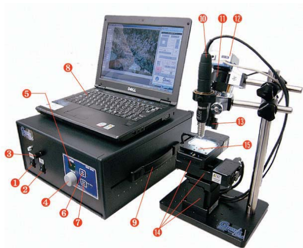
Fig. 1. High-precision micromilling system GEOMILL326. 1) Main power switch, 2) Power switch of LED light for CMOS-system, 3) LED light intensity control, 4-5) Micro motor speed control of micro drill, 6) Power switch of micro motor, 7) switch of drill rotation direction, 8) Computer for stepping-motor control of XYZ-stages and display of CMOS image. 9) Grip for carry, 10) Micro drill, 11) Zoom lens, 12) CMOS camera, 13) LED light, 14) Stepping-motor drive stages for XYZ axis, 15) Sample table.
