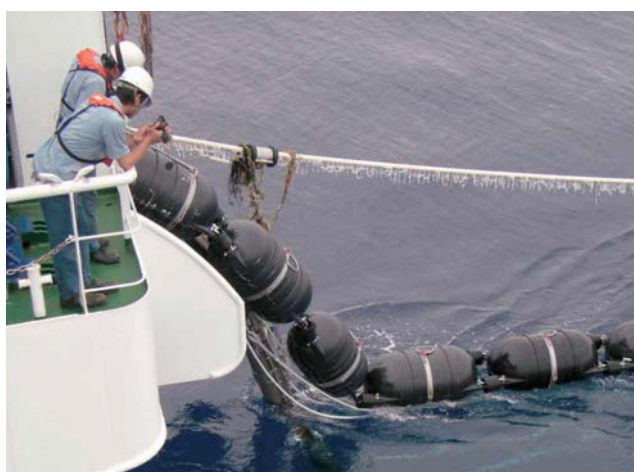
Fig. 3 Seismic System in Phase 5. (Top): Airguns of Kairei. (Bottom): Streamer cable.
