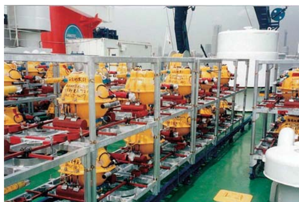
Fig. 2 Seismic systems in Phase 3. (Top): Airguns of Kairei. (Second from the top): Streamer cable of Kairei. (Second from the bottom): Airguns of Kaiyo. (Bottom): One hundred OBS on Kaiyo.
