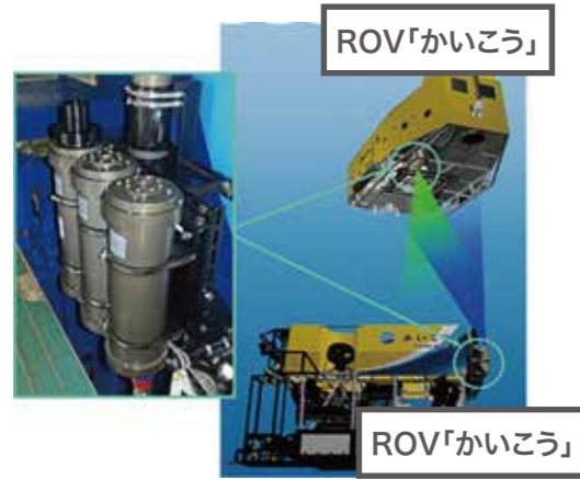
図3:レーザ通信装置 海域試験の模式図 ランチャー部とビークル部にそれぞれ水中光無線通信装置を搭載しお互いに同時に光を送受信して双方向通信を実施 Figure3: Bidirectional communication between an ROV launcher and a vehicle—both equipped with underwater wireless optical communication systems—simultaneously transmitting and receiving signals
