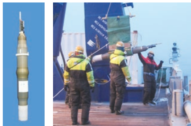
Fig.4 Deep-ocean profiling float "Deep NINJA" is deployed in the Antarctic Ocean from the R/V Mirai .
