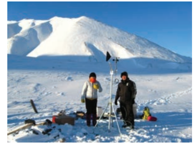
Fig. 8 Installation of automatic weather station in the Arctic mountain observation sites
