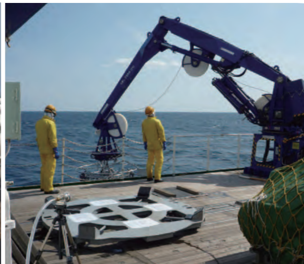
Water sampling operations. The sampler is lowered by crane and collects seawater. An apparatus that captures aerosol is mounted on the tripod at the bottom-left of the picture.
