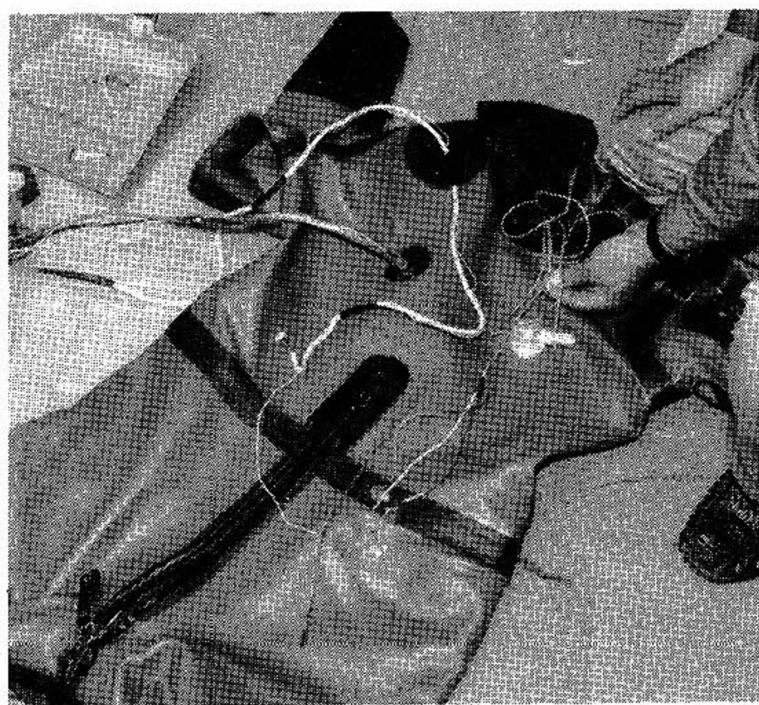
写真3 計測用コード Unbilical for measurement ; rectal temperature, 4 points skin temperature, heart rate
