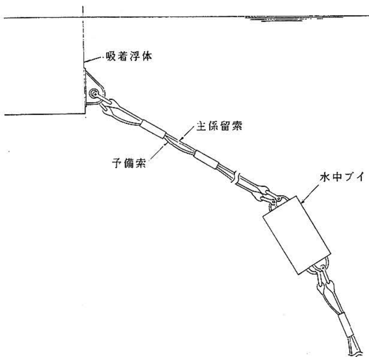
図7 係留索の破断対策
