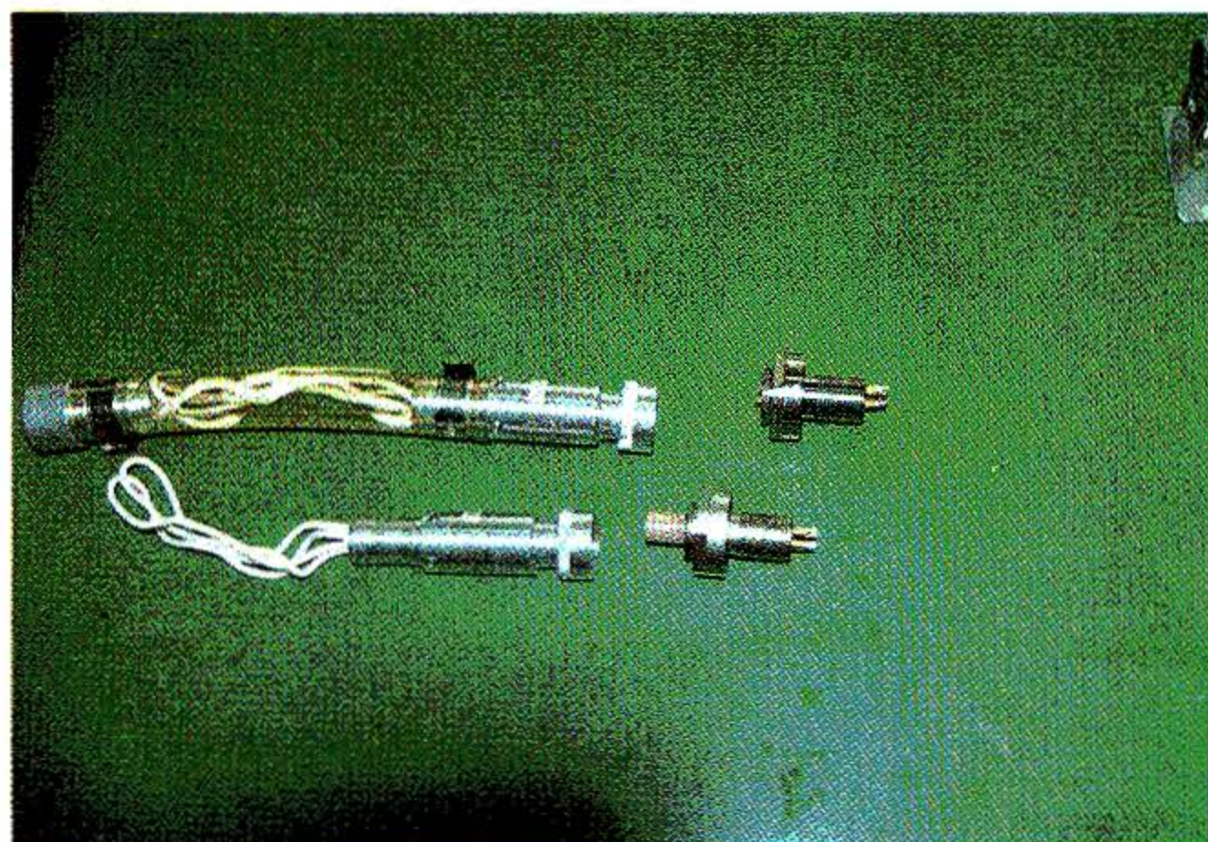
写真5 試作均圧型油漬コネクタ Photo 5 Oil filled connector as a model.
