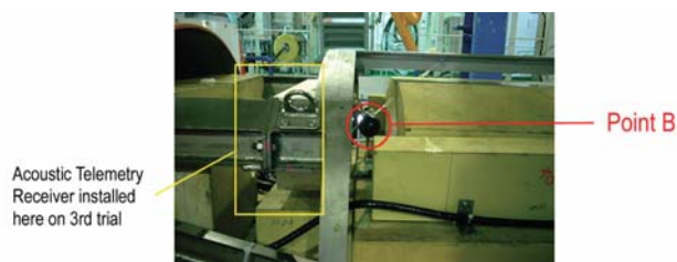
Photo 4 Hydrophone at point B on 4 th trial
