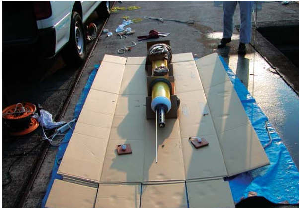
図10b 改良型緩衝容器に模擬フロートを収納する様子。右は緩衝容器底部に設置する緩衝材。 Fig. 10b The mock up laid on the unfolded improved container (left). A shock absorber installed in the bottom of the container (right).
