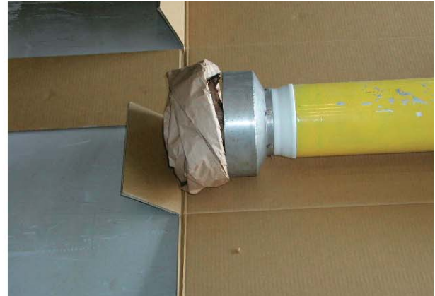
図10b 改良型緩衝容器に模擬フロートを収納する様子。右は緩衝容器底部に設置する緩衝材。 Fig. 10b The mock up laid on the unfolded improved container (left). A shock absorber installed in the bottom of the container (right).
