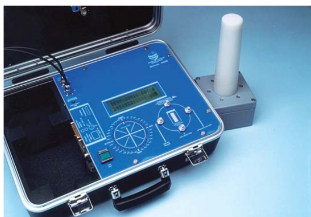
写真1 ARGOS方向探知器GONIO 400。本体(左)とアンテナ部(右)。 Photo 1 ARGOS direction finder GONIO 400. The main body (left) and the antenna (right).
