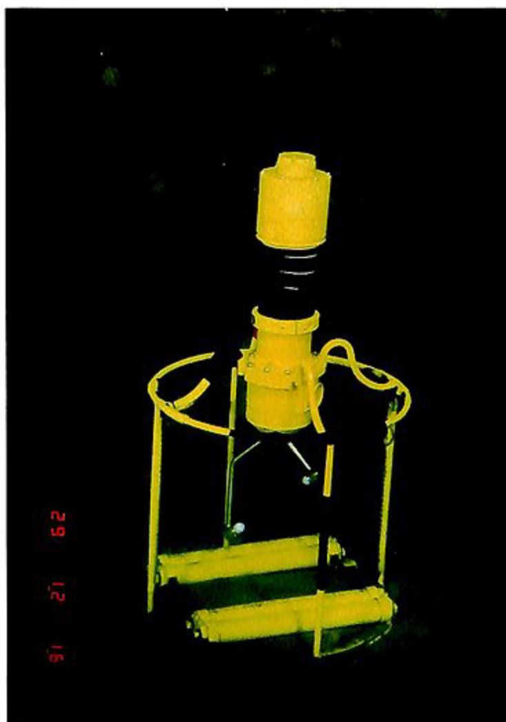
写真1 水深1961mの海底で作動中の流向流速計 The deep sea current meter operating at the sea bottom of the depth of 1961m.
