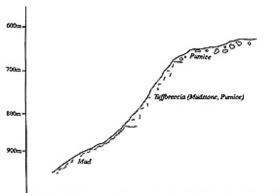
図5 Dive 539に沿った第五徳之島海丘の地層断面図 Fig. 5 Annotated profile of Daigo-Tokunosima Knoll along Dive 539.
