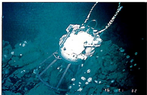
Photo 1 OBS/H deployed by the free-fall mode found at the first site. It was sandwiched by two rock slabs. The white ones are a kind of sponge.
