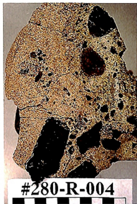
Photo 5 Photograph of a piece of foraminiferal limestone obtained on dive 280 containing swirls of green serpentine mud (right side of photo) and several small clasts of serpentinized ultramafic rocks (dark fragments). The scale bar at the bottom of the photograph is graduated in centimeter intervals.
