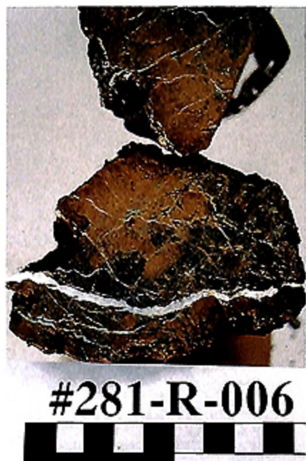
Photo 10 Fragment of serpentinized harzburgite that has been fractured and veined with carbonate. The scale bar at the bottom of the photograph is graduated in centimeter intervals. Veins in the sample are pure carbonate. Because they lack serpentine mud, it is thought that the rock was fractured before or during transport and was infiltrated with fluids from depth that caused precipitation of carbonate.
