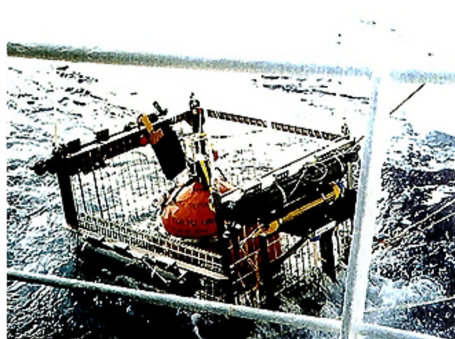
Photo 3 The deployment of the long-term OBS (#550) using the shuttle elevator.
