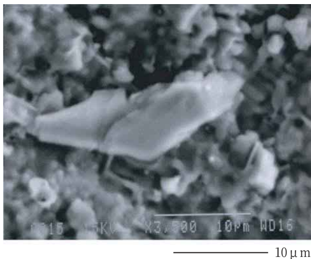
Fig. 5 SEM photograph of 2K#1179-R1 (burrow). The rhombic shape of authigenic dolomite is clearly observed.
