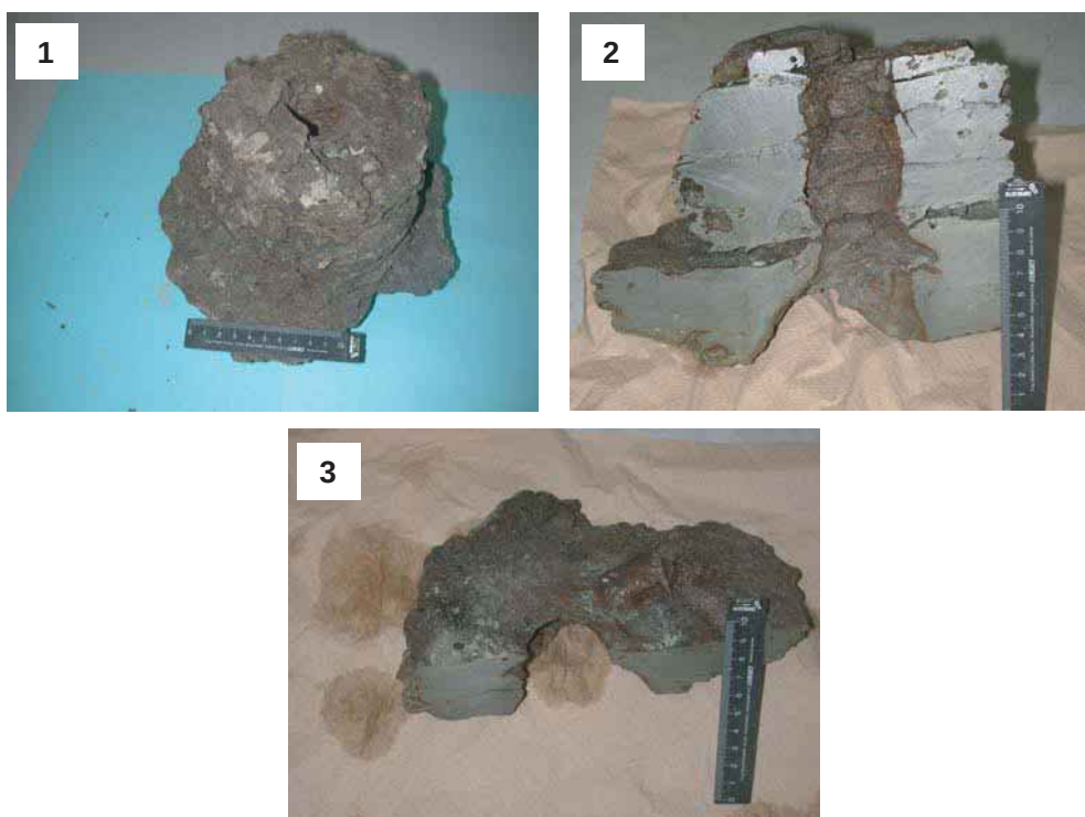
Fig. 4 Doughnut type originates in another chimney. 1 : Sample 2K#1264-R2 is big cylindrical. The diameter is about 15cm. The diameter of its vent hole is 3.5cm and not clogged. 2 : It was half-sized by a cutter. In the position of one thirds from below, the crack reach the vent hole. Spontaneously the lower part separates from the upper part. 3 : This photograph is the lower part. It seems like a doughnut type.
