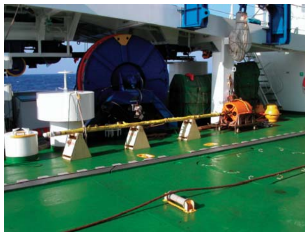
Fig. 5 Heat flow meter (HF) deployed in KR02-10.
