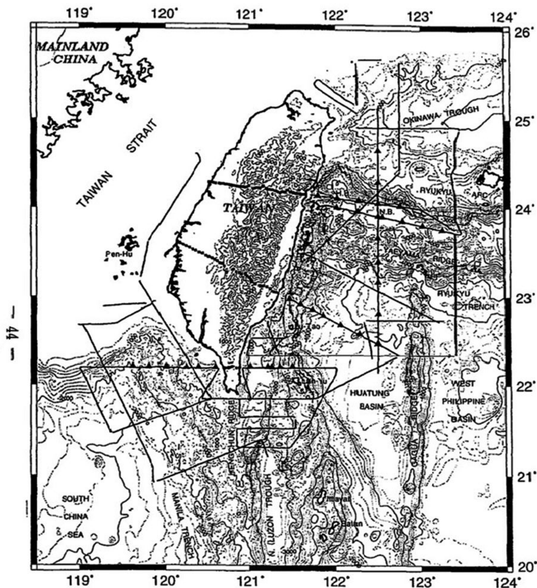
Figure 1. Map showing locations of the TAICRUST deep seismic reflection profiles (dark lines), ocean bottom seismometers (triangles) and land seismometers (squares). Bathymetric contours are in 200 meters.
